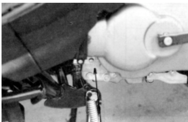
Location of Engine Serial Number
